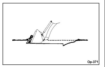
Make additional passes until desired depth is reached. During each pass, use only bucket control while working depth. This will allow you to concentrate on controlling bucket angle to maintain a precise cut.
